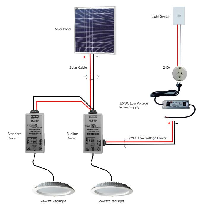
\*During the day if the light switch is in the off position both lights will be fed by the solar panel which in turn will respond to outside conditions. If full light is required, then simply turn the switch on for full powered light.
