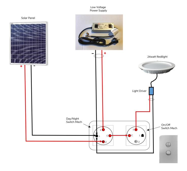
Note: The system above allows you to choose between a Solar or Grid supply for powering your light. An on/off is included for full control.
