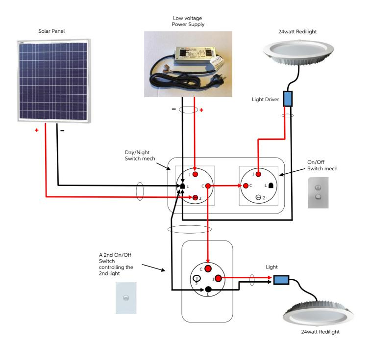
Note: The system above allows you to choose between a Solar or Grid supply for powering your light. Two On/Off switches to control lights individually.
