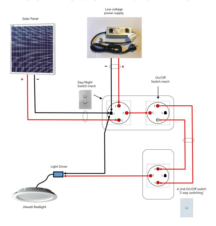
Note: The system above allows you to choose between a Solar or Grid supply for powering your light. This is a 2 way On/Off switching wiring diagram controlling one light.
