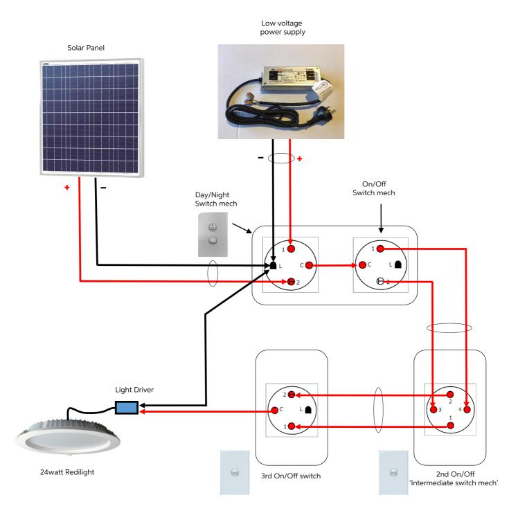
Note: The system above allows you to choose between a Solar or Grid supply for powering your light. This is a 3 way On/Off switching wiring diagram controlling one light.
