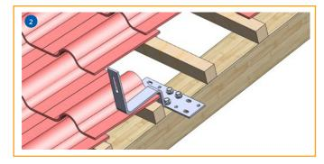
Tip: If the tile bracket is making the tile sit up you can do two things - use a pair of pliers to pinch out some tile on the underside in line with the bracket, OR use a grinder to trim a small section so the tile will sit snugly over the bracket.
