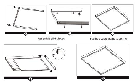
4. Unscrew one end of frame and remove, slide Skyfixture panel into frame then re-screw end back to frame.
