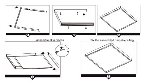
4. Remove one end of frame, slide the Skyfixture panel into frame then reinsert end back to frame
