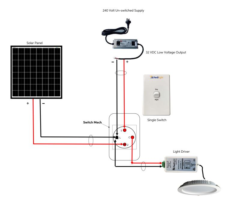
Note: When the switch is in the "DAY" position the light is powered by the solar panel. When switched to "NIGHT" the light receives full power provided by the low voltage power supply.
