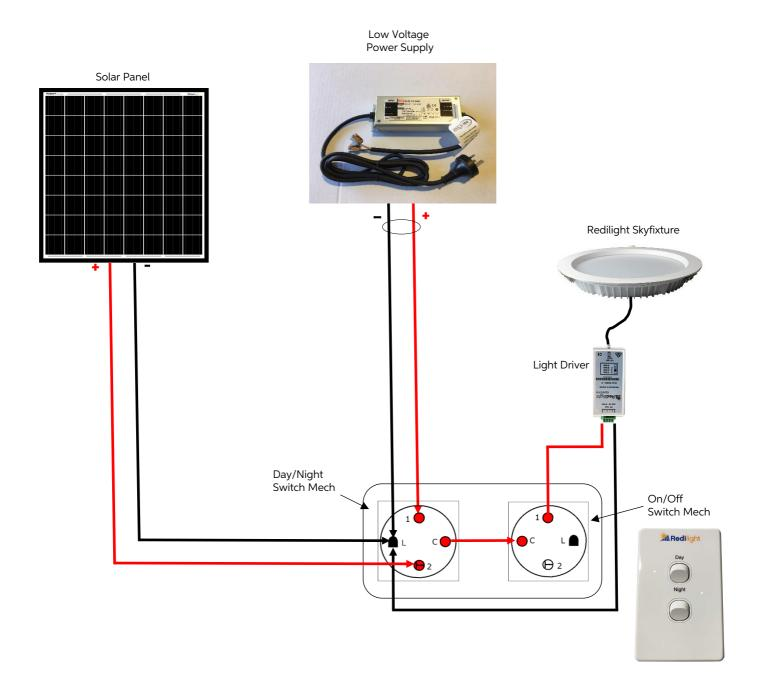
Note: The system above allows you to choose between a Solar or Grid supply for powering your Skyfixture. An on/off is included for full control.
