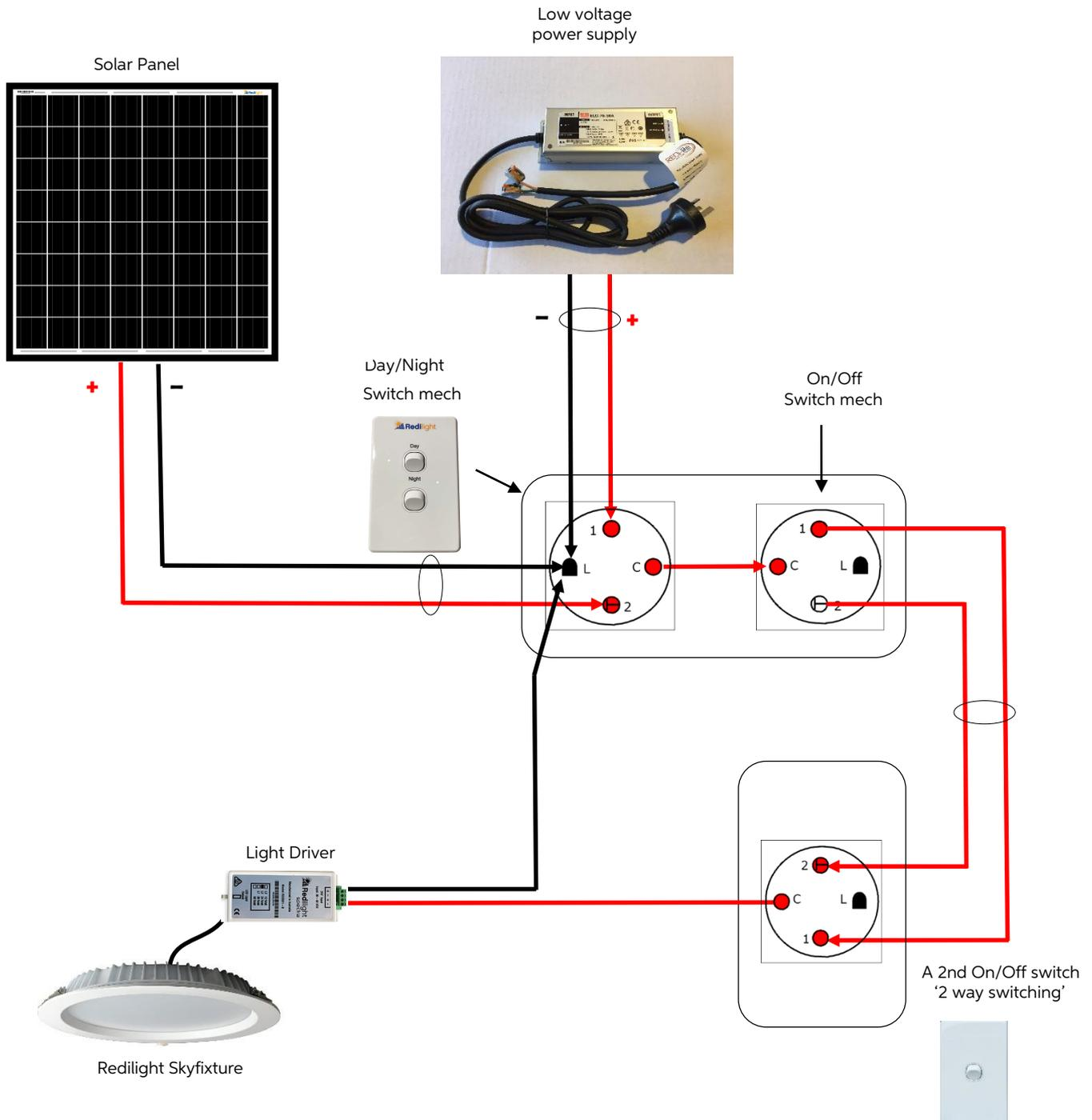
**Note:** The system above allows you to choose between a Solar or Grid supply for powering your Skyfixture. This is a 2 way On/Off switching wiring diagram controlling one Skyfixture.
