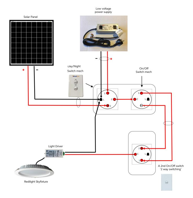
Note: The system above allows you to choose between a Solar or Grid supply for powering your Skyfixture. This is a 2 way On/Off switching wiring diagram controlling one Skyfixture.
