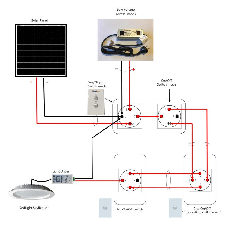
Note: The system above allows you to choose between a Solar or Grid supply for powering your Skyfixture. This is a 3 way On/Off switching wiring diagram controlling one Skyfixture.
