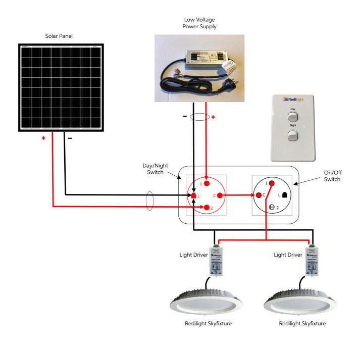
Note: The system above allows you to choose between a Solar or Grid supply for powering your light. One On/Off switch controls both Skyfixtures
