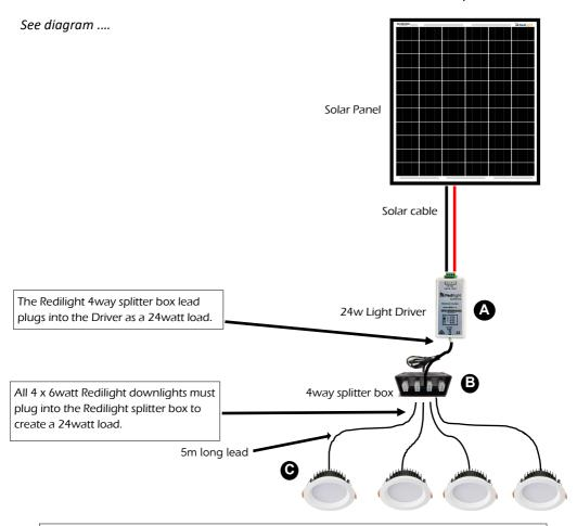
**CAUTION** - If On/Off control of the lights is required you must switch the driver which in turn controls the four lights. **Do Not individually switch each light fitting.**
